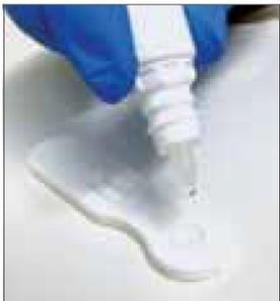
Hold the Buffer bottle vertically and 1cm above the circular well.
